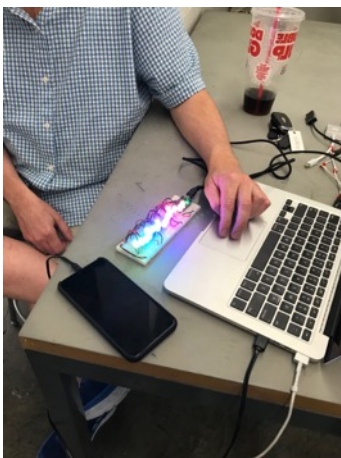
Programming a lighting sequence on a breadboard with RGB programmable LEDs
